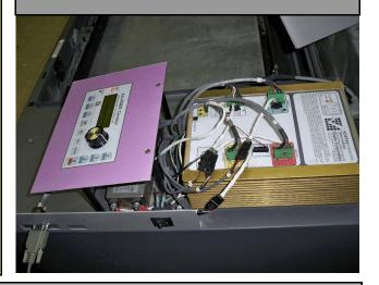
*SynchroStepping* \* All of our motion systems and drivers utilize a method that synchronously, microstep, sample and correct the current on multiple motor windings at a 20-50 kHz rate resulting in stable, quiet, smooth control of a stepper motor.
